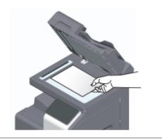
26. The bizhub C250i also contains an RADF with a document tray where original documents can be stacked to be scanned, and an output tray that receives the original documents output after scanning.
