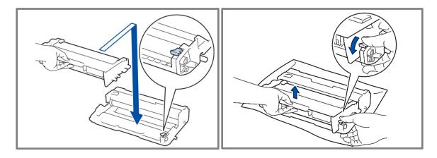
35. The IUP37 has a displacement mechanism activated by the lock lever. When the lock lever is pressed, the toner cartridge (toner replenishing container) comes out (is displaced) from the grooves of the IUP37 (container holding member) holding the toner cartridge (toner replenishing container).
